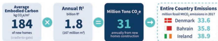
The CO 2 e from construction of new homes in the US is similar to the entire emissions of Denmark.
